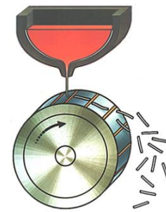
Figure 1. Diagram showing the hyperquenching process to produce the amorphous metallic fibres
