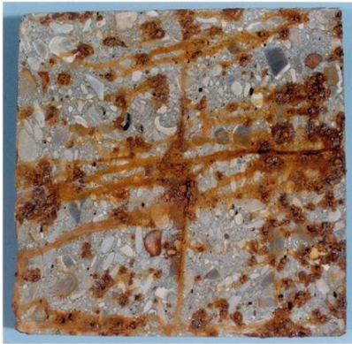
Concrete containing steel wires Aspect after 3 months
